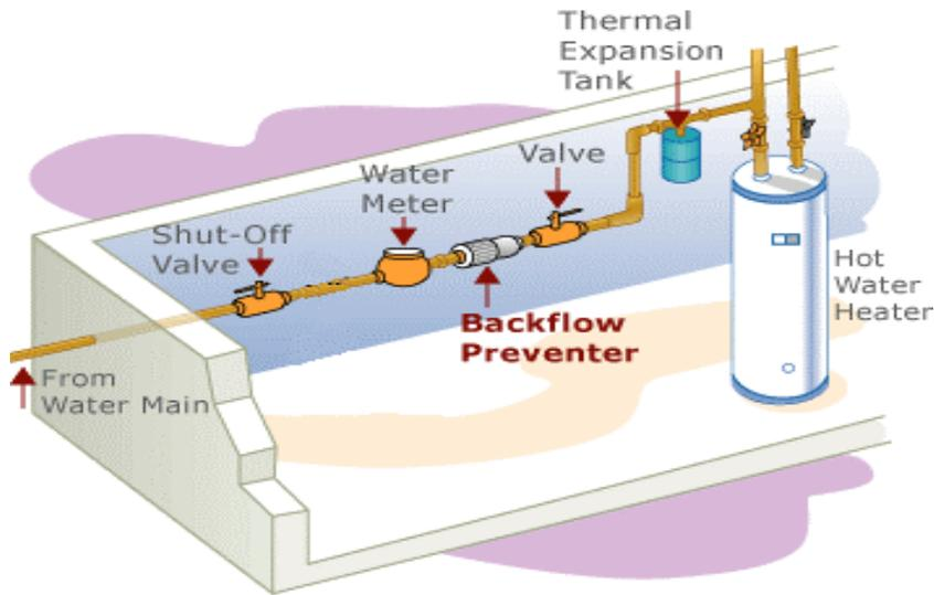
Many industrial and commercial customers on use water in manufacturing, in their heating or cooling system, or for other non-drinking uses. These customers are required to install a “backflow prevention device” where the water enters their building to prevent any possible contamination of the water mains. These devices are tested annually to make sure that they are working properly.
